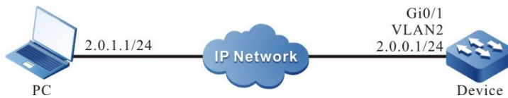
Figure 2-5 Network Topology for Configuring a Local Terminal to Telnet to the Device
